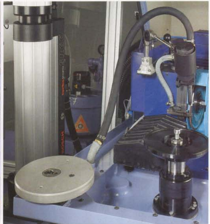
Automatic clamping of the saw blade
