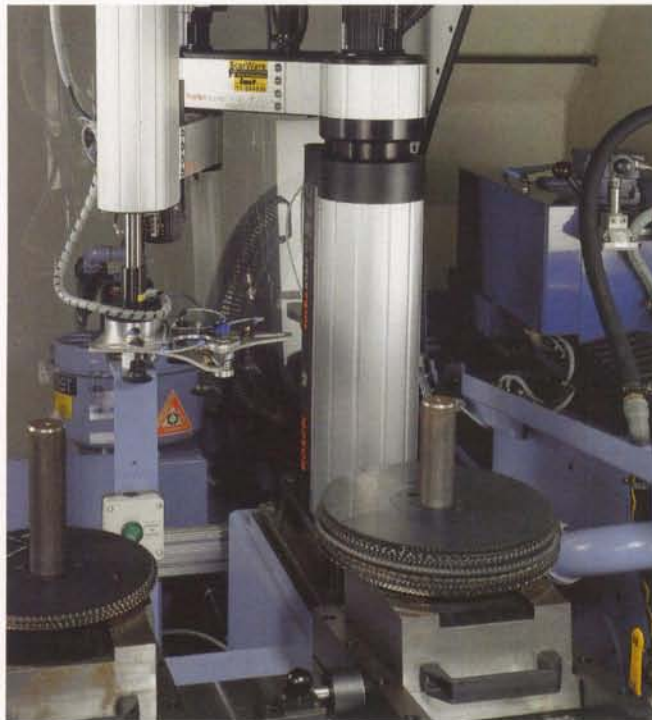
Raw material and finished product magazine, each having a capacity of 180 mm. Industrial robot for the handling of saw blades.
